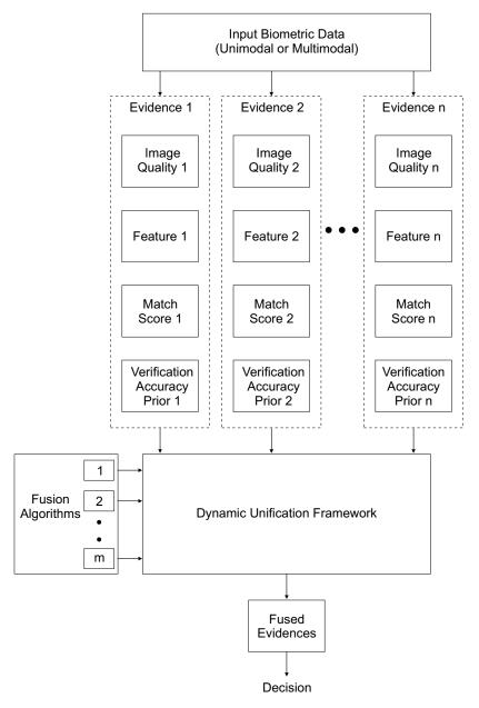
Fig. 1. General concept of the proposed unification framework.
