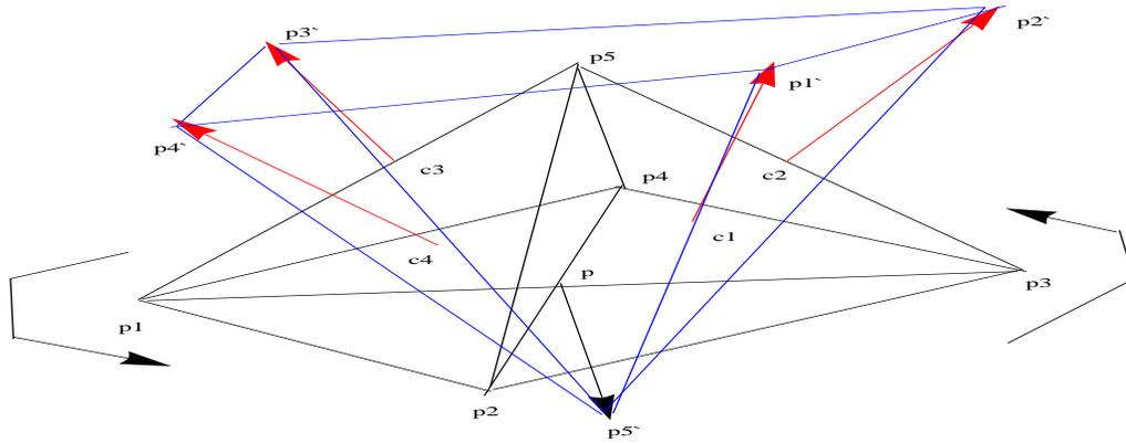
**Fig.3** Transformation of a pentahedron using method (4)
