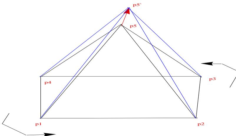
**Fig.2** Transformation of a pentahedron using method (3)
