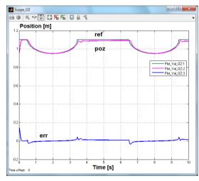
Figure 7 – Robot's foot positioning on OZ axis using RNC method
