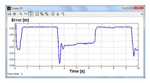
Figure 8 – Positioning error for leg 1 on OX axis using RNC method
