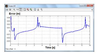
Figure 9 - Positioning error for leg 1 on OZ axis using RNC method
