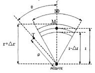
Fig. 1: Ultrasonic sensor model
