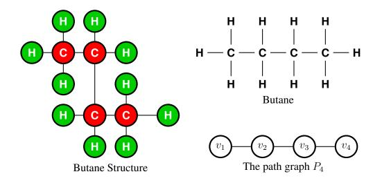
Suppose we can consider hydrogen detected graph  $P_4$  as in Nover top graph structure, we can calculate the Nover top  $Z_1$  index for  $P_4$ . Hence the boiling point of butane in Nover top graph is satisfies linear equation as  $t_B = aW + bP + c$ . Since butane is non-polar, b = 0. so,  $t_B = aW + c$ . If we can take for particular value of a, b, c and get the boiling point of butane both of them is same.
