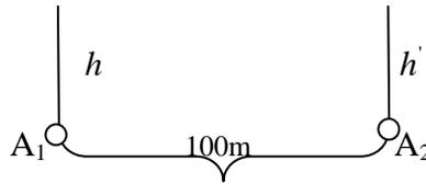
**Determining the distance using the sound speed and binoculars.**
