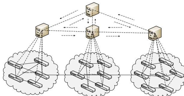
Figure 1. Hierarchical SDN structure.
