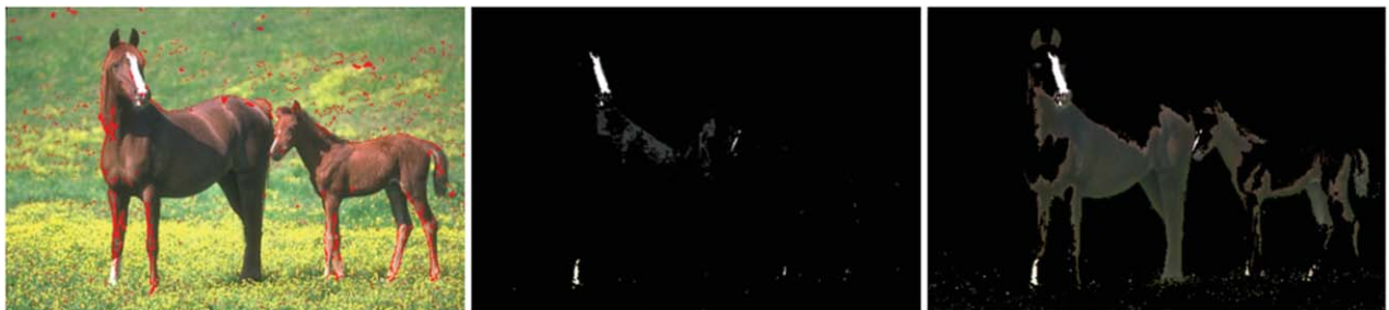
Fig. 5. Composite image of three segmented colors (left) and results obtained with the old (center) and the new achromatic zone G (right).
