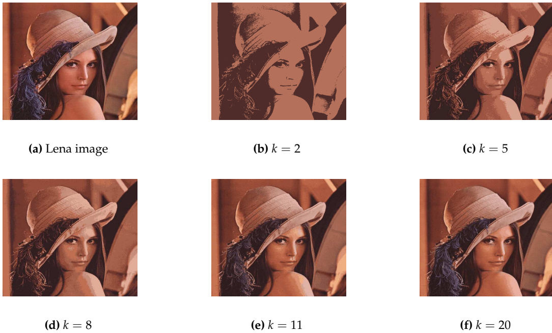
Figure 2. The image segmentation for Lena image. (a) the original Lena image (b-f) the clustering images when the number of clustering k = 2, 5, 8, 11 and 20 respectively.
