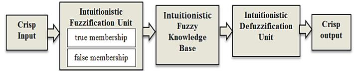
Figure 2: Block Diagram of Intuitionistic Fuzzy Inference System
