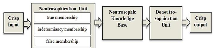
Figure 3: Block Diagram of Neutrosophic Inference System
