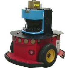
Fig.1. Pioneer 2-DXe mobile robot
