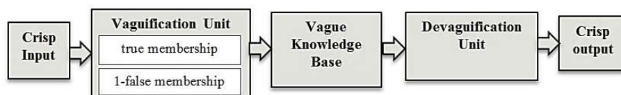
Figure 3. Block Diagram of Vague Inference System
