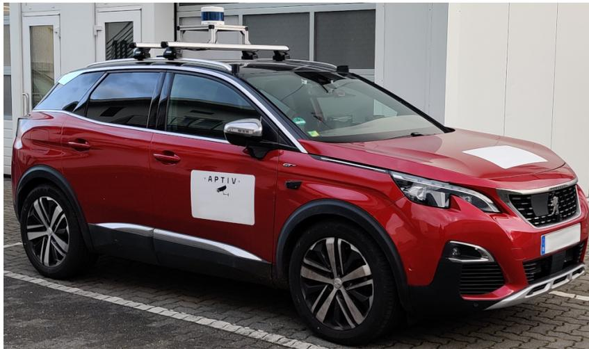
**Figure 7.1.** Experimental vehicle Peugeot 3008 used to test capabilities of presented algorithm. Vehicle is equipped with four corner radars and reference camera system. High resolution LIDAR visible on the roof was disabled for presented experiments.
