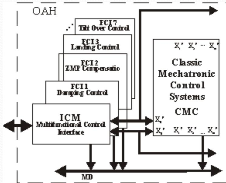
The HFPC system was designed with an open architecture (OAH) in a distributed and decentralized structure to enable easy development of new applications or adding new hardware modules or software for new control functions.
