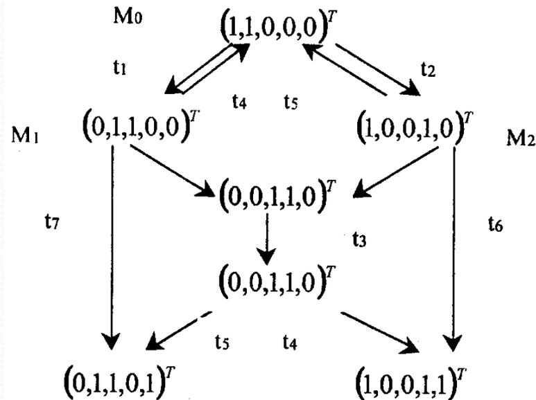
Associated Markov graph of the system modeled by means of Petri nets
