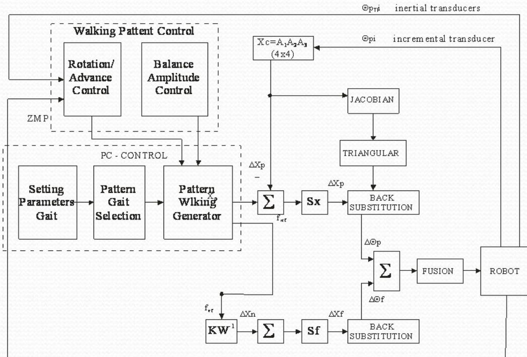
**The walking pattern control**, may be changed periodically according to the information received from an inertia transducer during each walking cycle.
