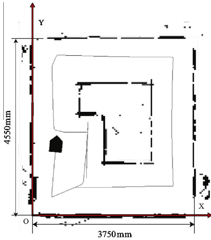
Fig. 7. Map building based on GFM after improving the sonar model.
