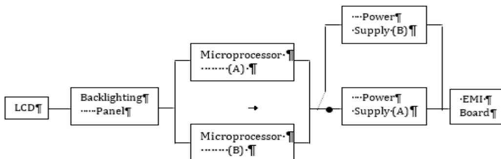
Figure2. LCD display unit
