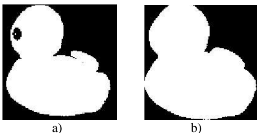
Fig.2: Applying the dilation operator: a) the Original binary image b) the dilated image.
