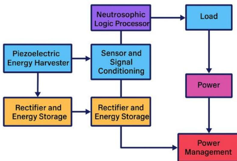
**Figure 12: Block Diagram of a Power Management System for Energy Harvesting with Neutrosophic Logic**
