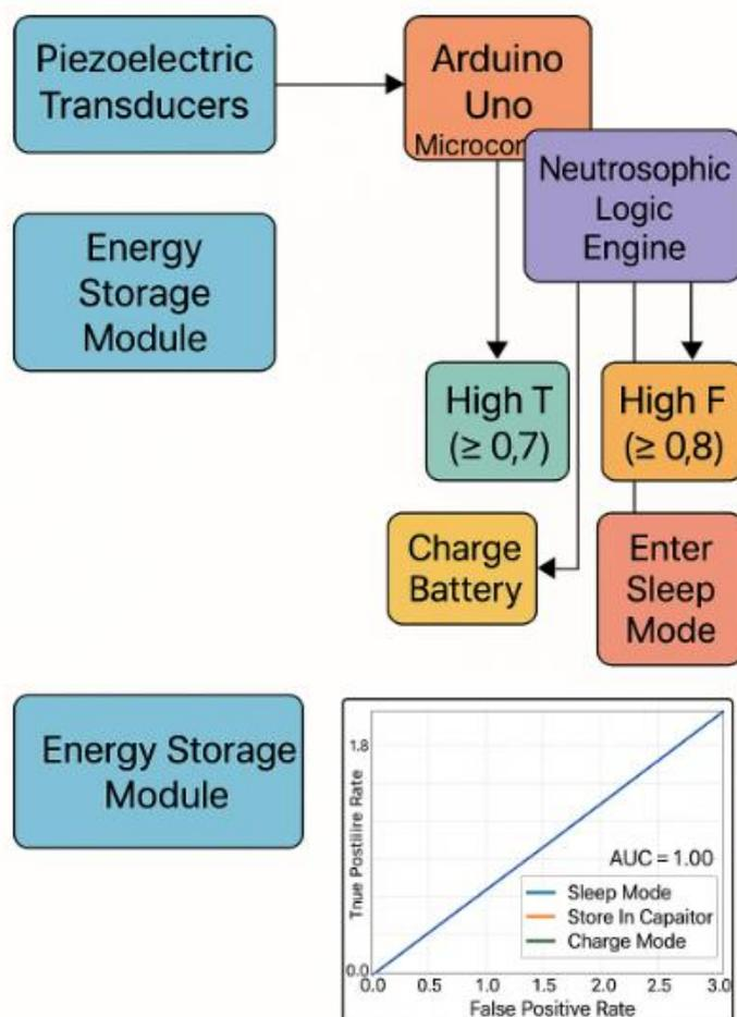
This flowchart represents the operational sequence of a piezoelectric energy harvesting (PEH) system enhanced with neutrosophic logic-based decision-making. The methodology consists of four primary stages:
