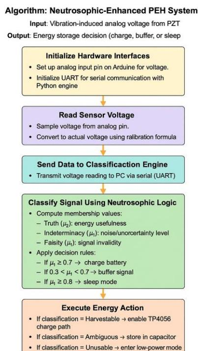
Figure 4: Algorithmic Workflow of the Neutrosophic-Enhanced Piezoelectric Energy Harvesting (PEH) System
